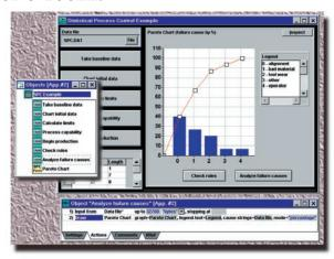
The Statistical Process Control (SPC) Toolkit charts process data in real time, automatically derives control limits from your data, monitors process quality, tests for limit violations or trends, and produces standard SPC charts.
