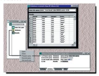
The Database Toolkit allows direct access to all popular database packages right from TestPoint, with no low-level coding, or exporting and importing of disk files. This lets you store measurement and test results or retrieve configuration information.
