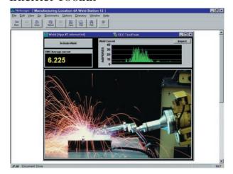
The Internet Toolkit provides the ability to view and control remote applications using an internet browser or TestPoint application. Remote sites can send email based on test status, or can communicate directly with any TCP/IP network client.
